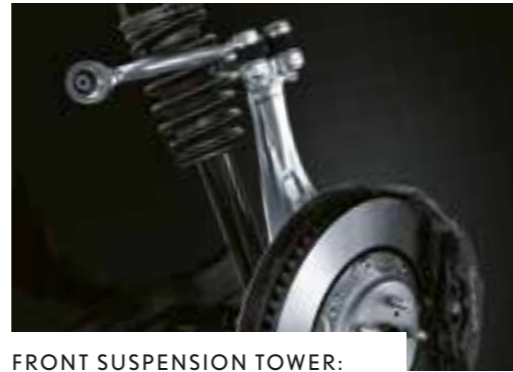
FRONT SUSPENSION TOWER: ALUMINIUM
