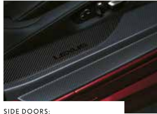
SIDE DOORS: OUTER - ALUMINIUM INNER - CARBON FIBRE
