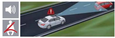
Third warning: At this stage, there's a chance that a collision will occur. The CMBS system starts emergency braking and activates the brake assist function to reduce speed. At the same time the seatbelt tightens to reduce the impact of the collision on the driver and front passenger.
