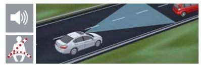
Secondary warning: If the distance between the two vehicles continues to decrease, CMBS applies light braking and the seatbelt E-pretensioners in the driver's side gently pull two or three times. At this point the E-pretensioners pull the seatbelts with enough force to properly restrain you and your front passenger, giving you time to react and avoid a collision.
